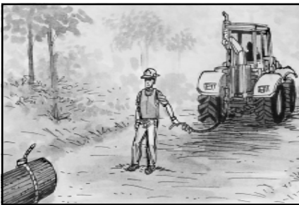
c. Enganche del cable principal
